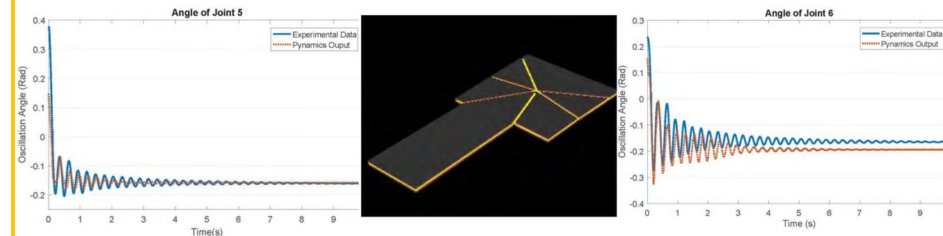
The output of Pynamics is in the form of graphs of position, velocity and acceleration of the bodies as well as animation of the moving mechanism
