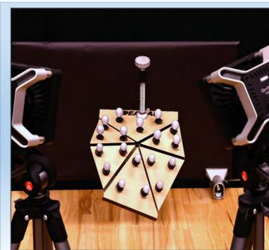
The dynamics of a laminate mechanism is recorded using OptiTrack cameras.
